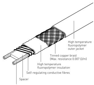
Electrical heat-tracing for process temperature maintenance applications up to 150°C which may be subject to steam cleaning.
