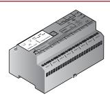
The Raychem NGC-40 works with the MONI-RMM2 module. Each RMM2 module installed in the field can accept up to 8 RTDs. 16 RMM2 Modules can be daisy chained together via RS-485 for a total of 128 temperature inputs. Since multiple RMM2s can be networked over a single cable to the Raychem NGC-40, the cost of RTD field wiring will be significantly reduced.
